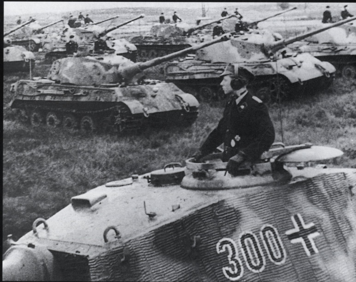
SS King Tigers in Hungary, 1945. Introduced at the end of 1944, the King Tiger was the best-protected tank of the war, and its long 8.8-cm gun could destroy any Allied tank at ranges of up to 2000m (6562ft).
